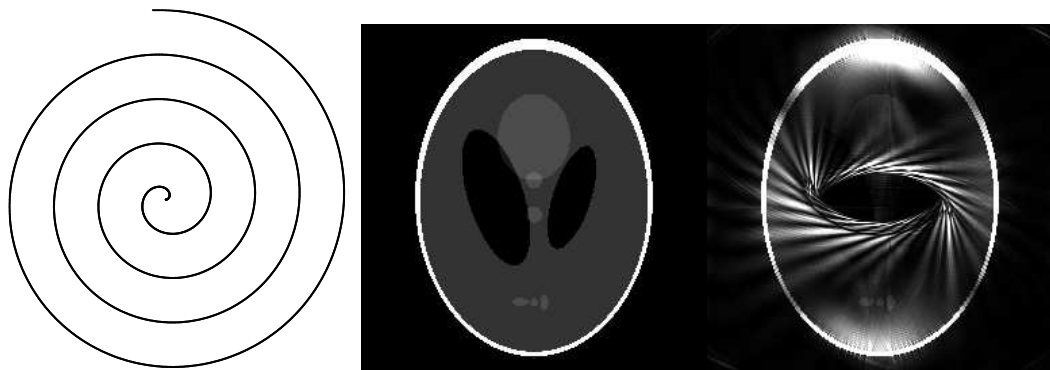
Figure 3.4: Left: 2D Spiral trajectory. Middle: Phantom image. Right sum of square image from each coil.
